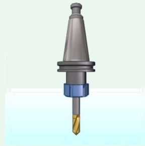
T2 Centerboor 12 mm S 3000 omw/min F 300 mm/min
