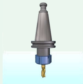
T8 Finishfrees 8 mm S 3750 omw/min F 500 mm/min
