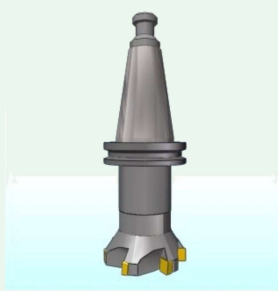
T1 Vlakfrees 63 mm S 3000 omw/min F 750 mm/min
